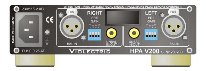
When a cinch plug is inserted, it cuts possible signals applied to the balanced input automatically. I.e. the cinch input has *priority*. Input impedance for all inputs is 10 kohms. Maximum input level should not exceed +21 dBu. This value is reduced to +15/+9 dBu if **PRE-GAIN** is set to +6/+12 dB !!
